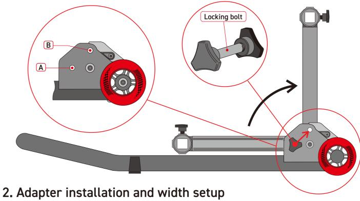
To install or adjust the adapter unscrew the adapter locking bolt and insert the adapter. The depth of the adapter can be adjusted to fit width of specific motorcycle.
